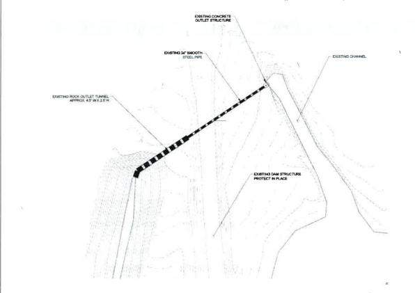
This project will address several problems to keep the reservoir working. First, the channel preceeding the outlet will be shored up with concrete wingwalls and backfilled to prevent collapse. The outlet itslef will be replaced and reinforced with a rock check dam. The pipe within embankment that is currently steel (first section) and rock (section section) will be replaced with precast concrete (first section) and HDPE (second section). A new valve system will also be added.
